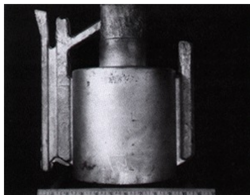
Fig 3.3a: Typical ZA-12 (zinc alloy) casting made from a plaster mould [436]
